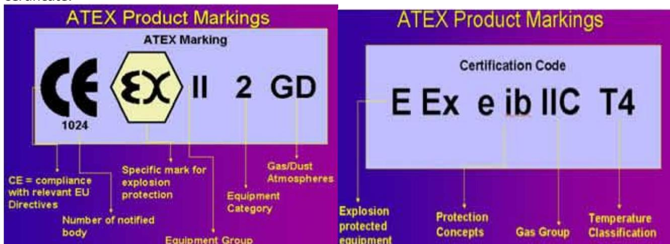
Equipment for use in explosive atmospheres should be regularly inspected and maintained to ensure it does not pose an increased risk of causing a fire or explosion. Maintenance of the equipment should only be carried out by people who are competent to do so. BS EN 60079 part 17: Explosive atmospheres. Electrical installations inspection and maintenance offers guidance as to the frequency and scope of maintenance required.
