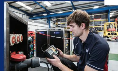
All IDE equipment is fully tested by our in house electricians before every hire. Equipment can be supplied to you with a valid test certificate upon request. We can also carry out annual testing on your equipment, and issue you with appropriate certification.
