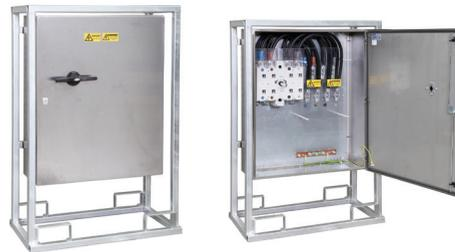
IDE manual changeover panels are designed to allow the user to manually divert the power to a secondary supply upon failure of the duty supply. Available 800A and housed in a stainless-steel crash frame.
