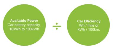
To calculate distance, use the formula: 'battery size in kWh' / 'Wh per mile'. E.g Renault Kangoo ZE, 31kWh battery, 265 Wh per mile, so 117 miles typical. Of course like a petrol or diesel car, range depends on how fast you drive, acceleration etc. Batteries are also affected by temperature, so on cold days range is less than warm days.
